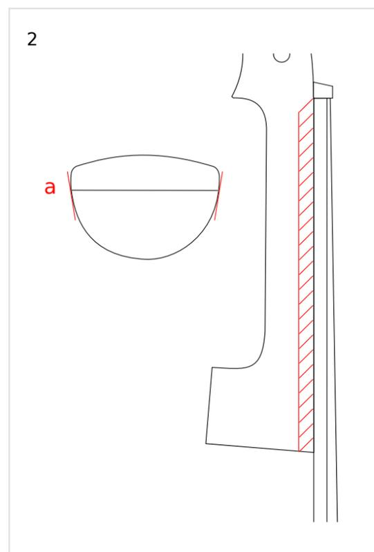
9. Along the length of the underside of the neck, scribe a parallel line at about 1/3 distance from the fingerboard, see Fig. 4. The same on the other side.
