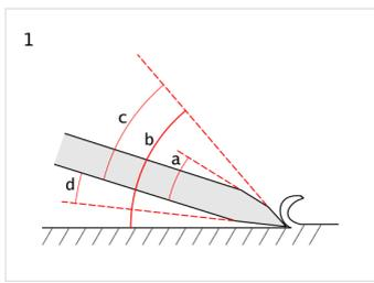
See Fig. 2 for the basic bevel down tool geometry. Bevel down tools include smoothing and jointer planes. "a" - Bevel angle, "b" - Cutting angle.
