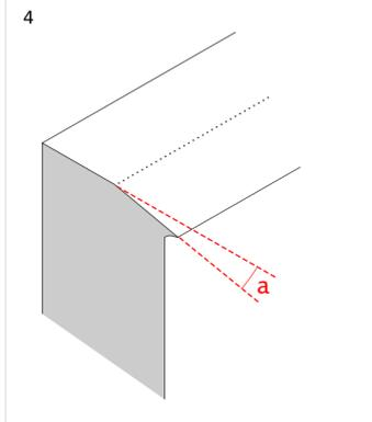
Cutting the denser sorts of wood requires blunter bevel angles, whereas softer woods allow for more sharply beveled tips. Ideally, the sharpest bevel should be employed which makes the tip still strong enough to withstand the pressure of the wood.
