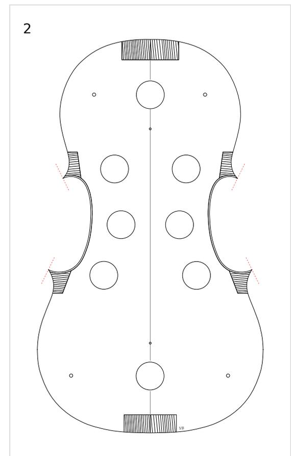
The top ribs can be made of two parts and there is no need to precisely pair them as with the bottom ribs. The ensuing gap at the top should not exceed 9 mm though. See the small gap at the top underneath the top clamping block in Fig. 2 for an example. Also see the exploded view in Fig. 1 to realize by how much the top and bottom ribs extend the feathered ends of the C ribs at this point to get an idea how long you should cut them before bending.
