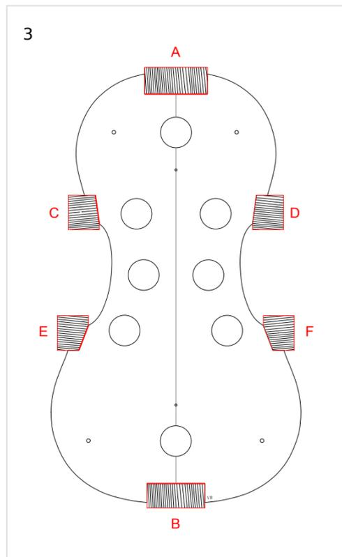
With most violins, the height of the ribs decreases gradually along the length of the body. Therefore, in the finished violin, the bottom block may be 32 mm tall, whereas the top block may be 30 mm in height. This, of course, affects the upper and lower cornerblocks as well. For Messiah, the final heights in the finished rib structure is as follows: A 30 mm , B 32 mm , C 30.5 mm , D 30.5 mm , E 31.5mm , F 31.5 mm .
