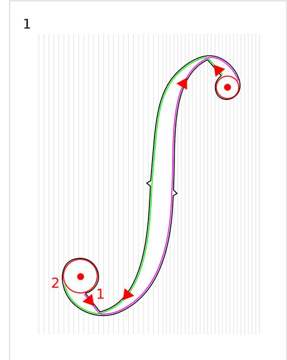
The angle of the f-hole walls depicted in Fig. 2. is more or less the modern standard and it can vary depending on the violin model. The gaps at the wing tips should have the width of about 1 mm .
